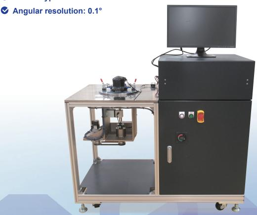
Unique mechanism design enables cogging torque measurement that suppresses the influence of cogging torque on the driving side of the external drive source.
