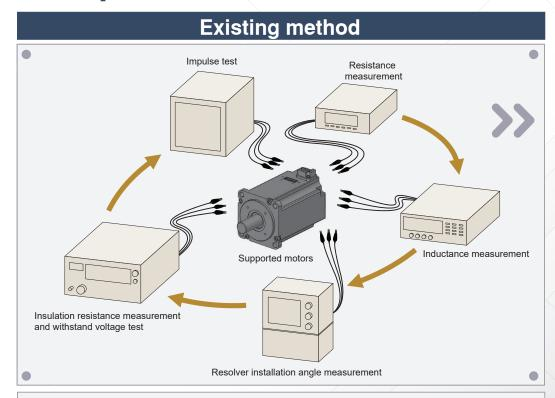
Wiring needs reinstalling for each measurement.
